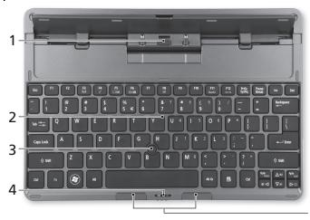
No. Item Description 1 Dock connector Connects to the tablet. 2 Keybaord A standard keyboard with full-size keys. 3 Acer FineTrack Pointing device to control cursor movement. pointing device 4 Secures the tablet to the docking station / Latch keyboard when closed. 5 Left and right buttons Function like the left and right mouse buttons.
