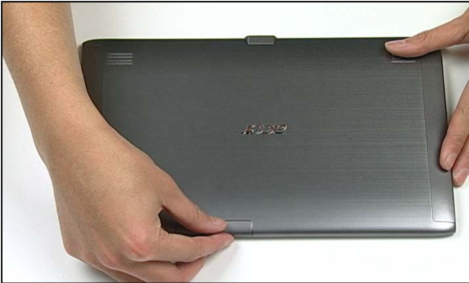
Figure 3-21. Securing SIM/Micro-SD Card Cover
