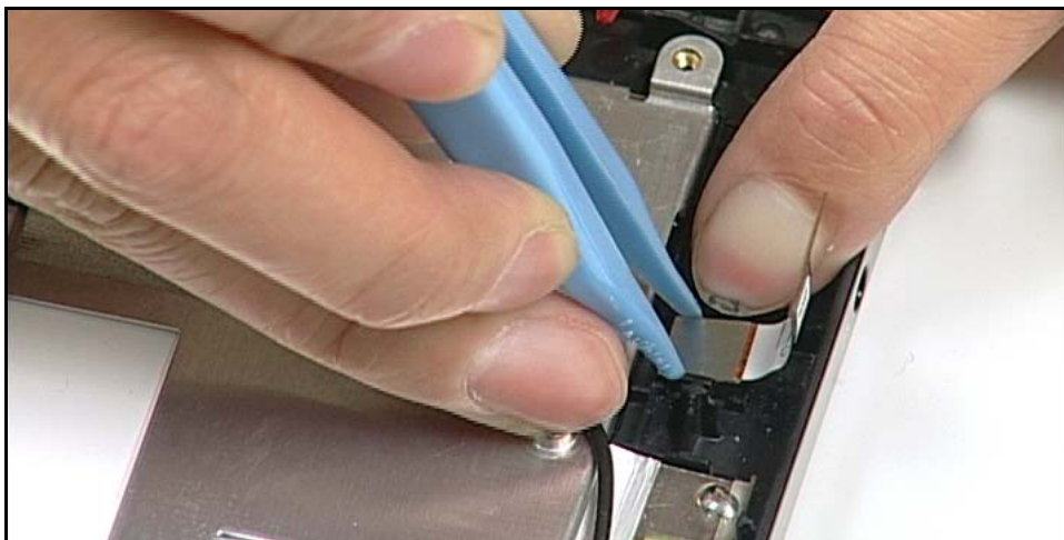
Figure 3-54. Removing Front CCD
