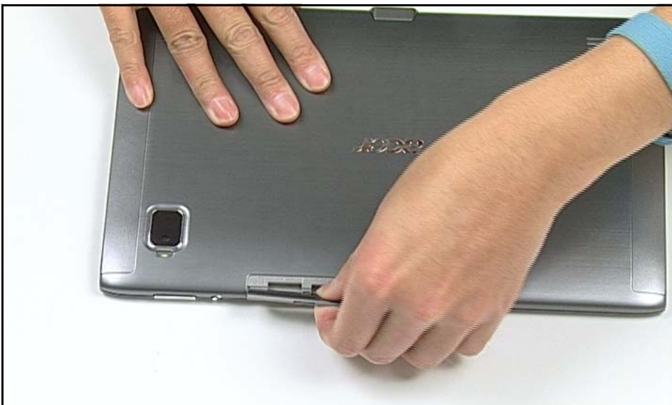
Figure 3-16. Installing Lower Case on Bezel
