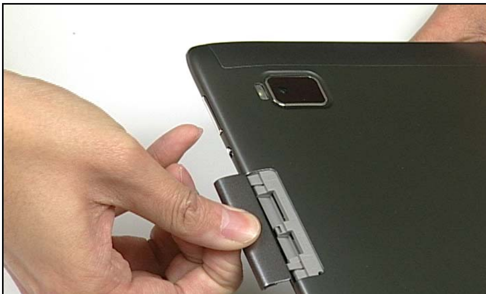
Figure 3-3. Opening SIM/Micro-SD Card Cover
