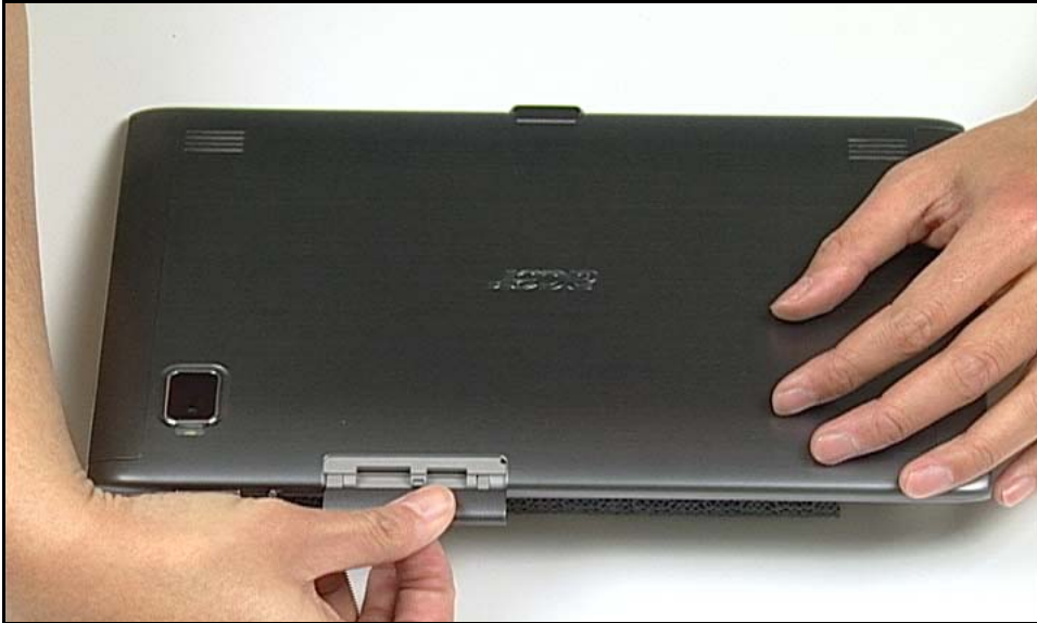
Figure 3-7. Opening SIM/Micro-SD Card Cover
