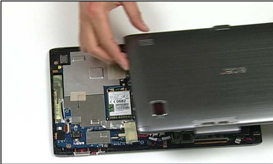
Figure 3-13. Removing Lower Case
