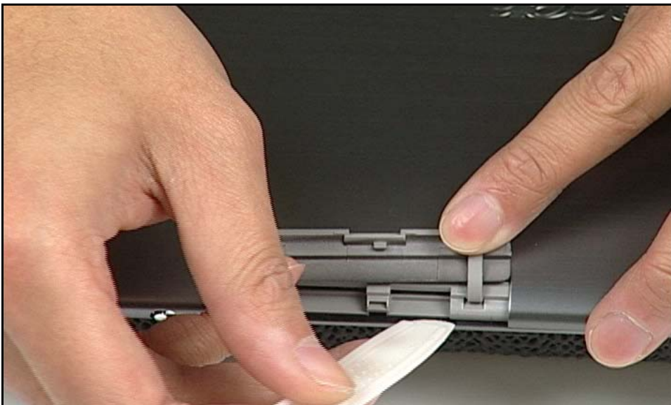
Figure 3-8. Unlocking Locking Latches (1 of 5)
