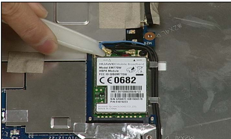
Figure 3-30. Disconnecting 3G Cables
