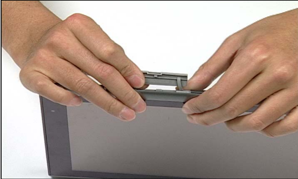
Figure 3-17. Securing Locking Latches (1 of 4)
