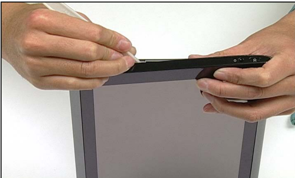
Figure 3-12. Unlocking Locking Latches (5 of 5)
