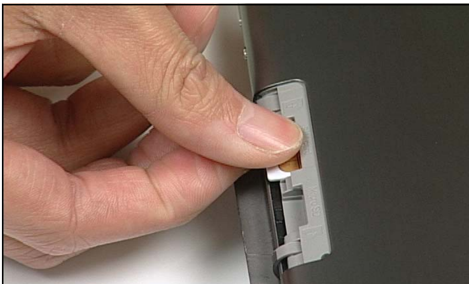
Figure 3-4. Removing SIM Card
