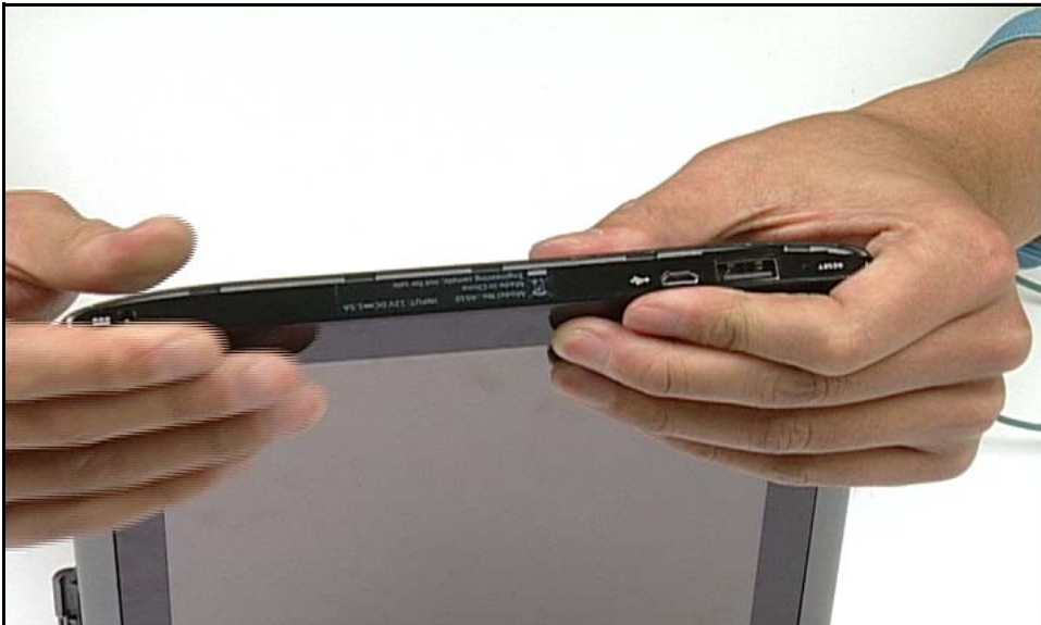
Figure 3-18. Securing Locking Latches (2 of 4)
