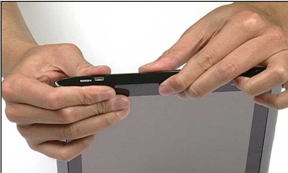
Figure 3-20. Securing Locking Latches (4 of 4)
