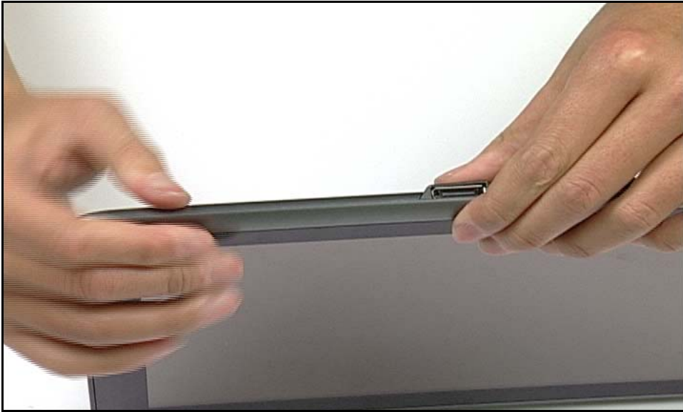
Figure 3-19. Securing Locking Latches (3 of 4)
