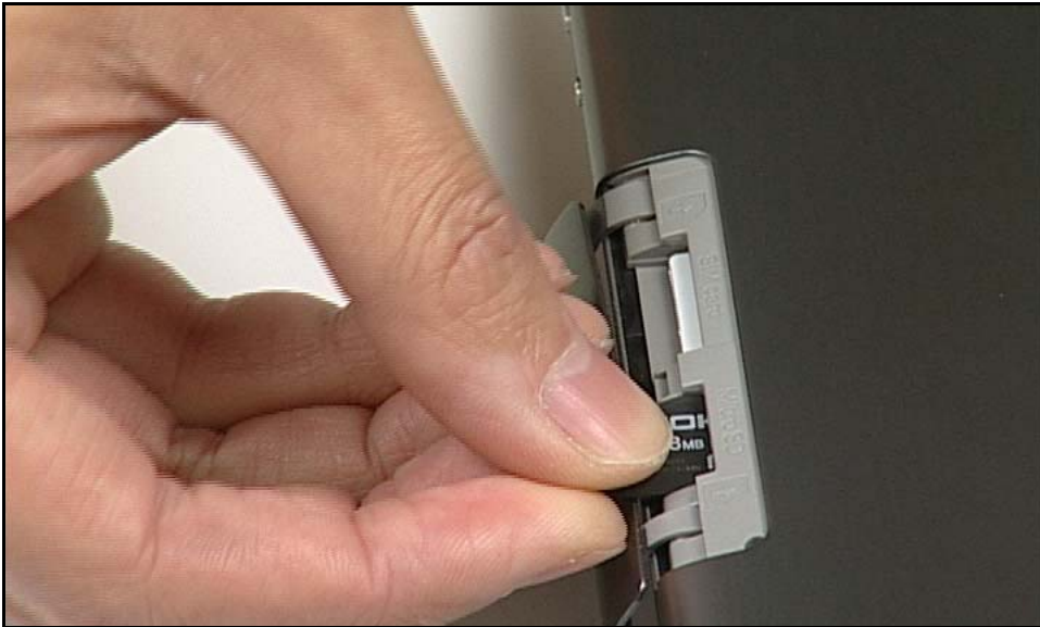
Figure 3-5. Removing Micro-SD Card
