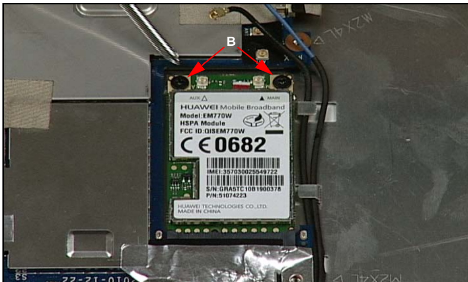
Figure 3-31. Removing 3G Module Screws
