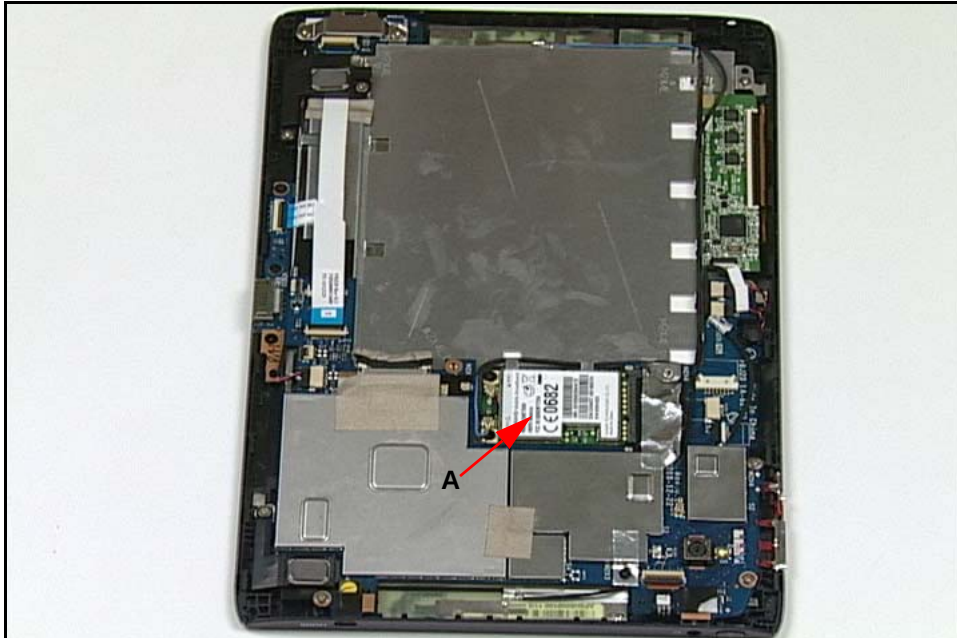
Figure 3-29. 3G Module on LCD Support Plate
