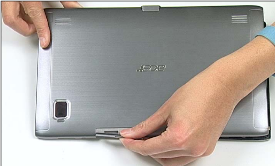
Figure 3-15. Aligning Lower Case with Bezel
