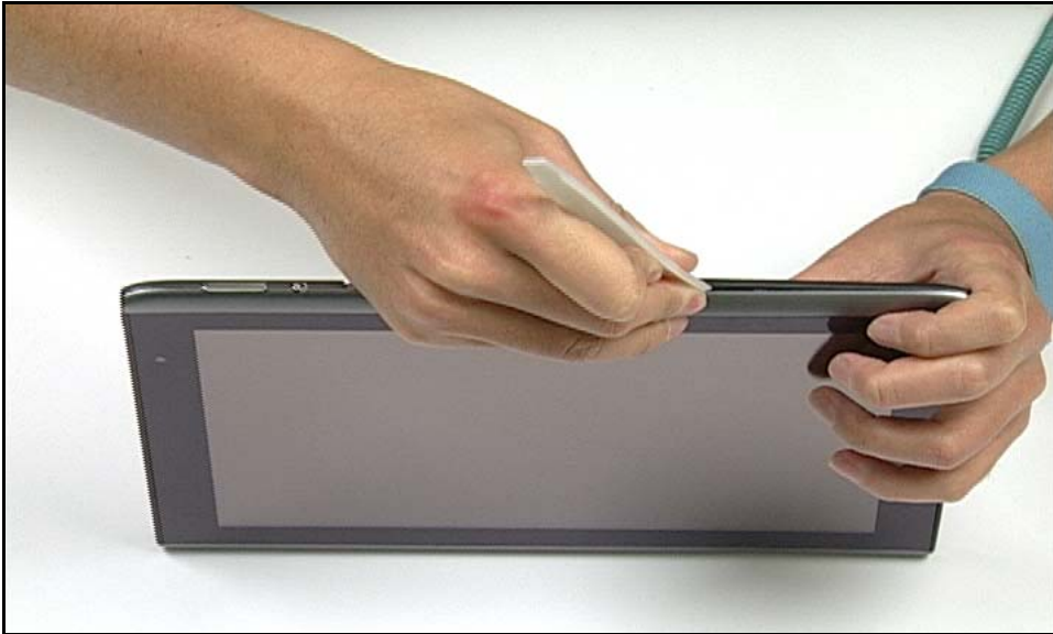
Figure 3-9. Unlocking Locking Latches (2 of 5)
