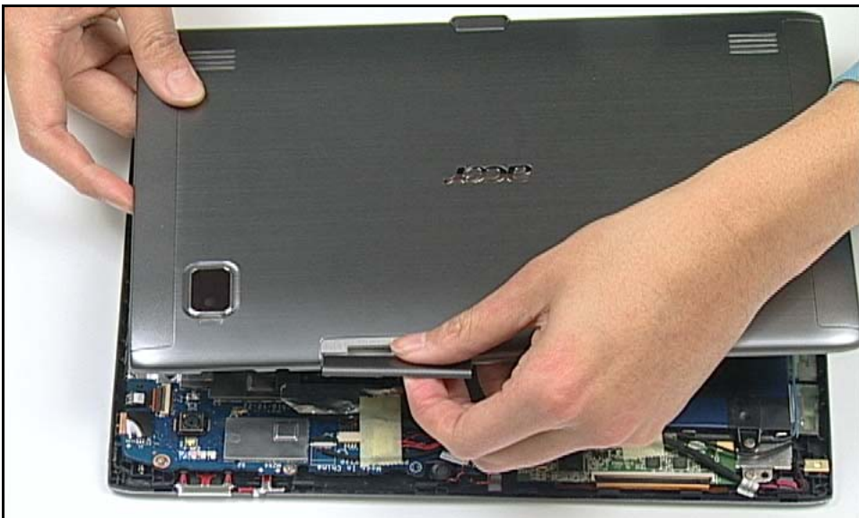
Figure 3-14. Opening SIM/Micro-SD Card Cover
