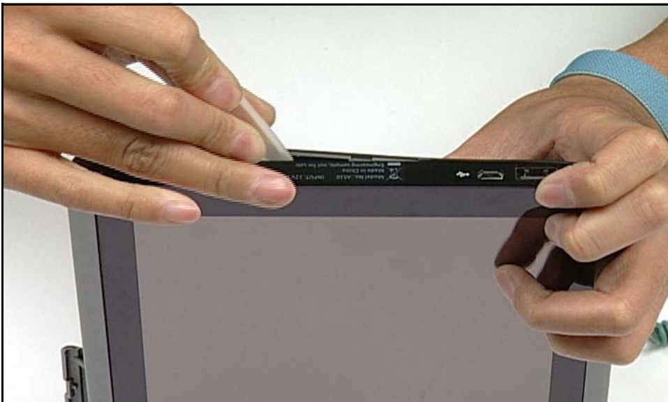
Figure 3-10. Unlocking Locking Latches (3 of 5)
