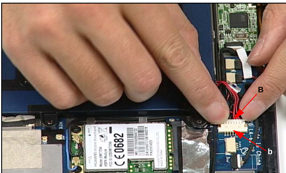
Figure 3-27. Disconnecting Battery Cable
