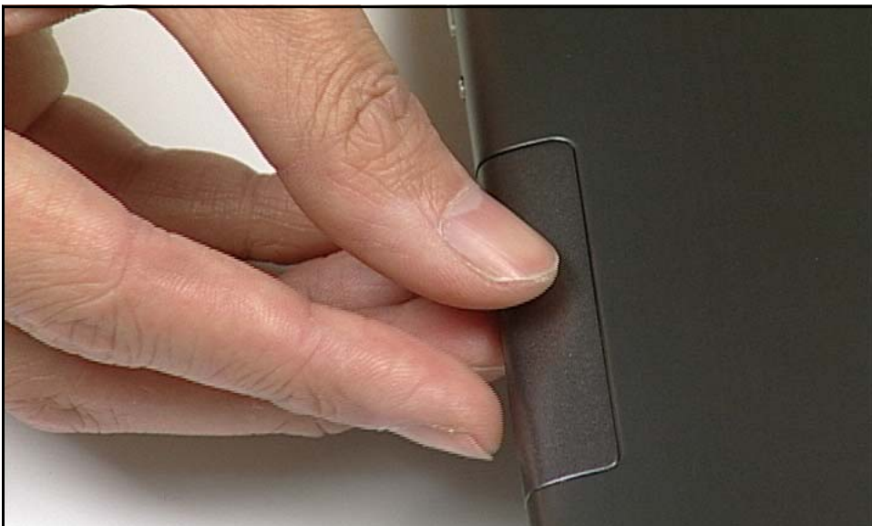
Figure 3-6. Securing SIM/Micro-SD Card Cover
