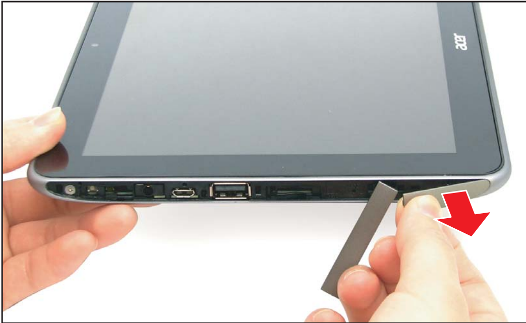
Figure 5-11. Unlocking the Left IO Cover Latches (4 of 4)
