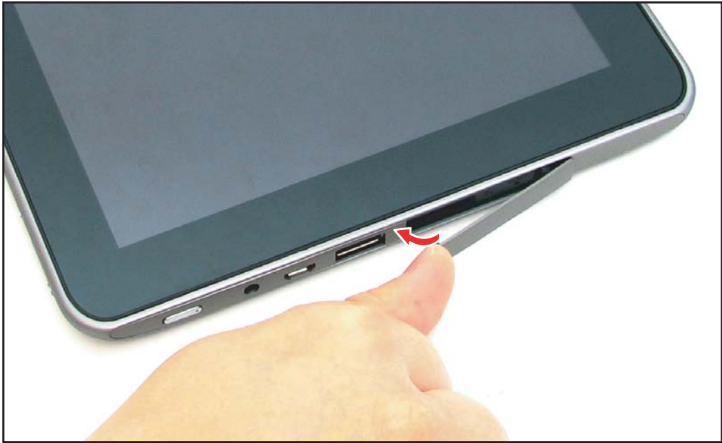
Figure 5-27. Closing the SD Card Cover
