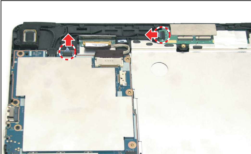
Figure 5-51. Disconnecting the Touch Panel Control Cable Connectors
