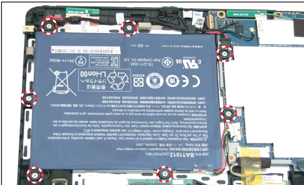
Figure 5-29. Removing the Battery Screws
