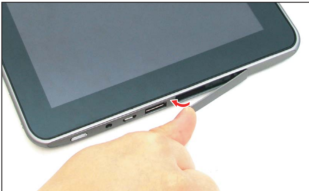
Figure 5-5. Securing the SD Card Cover
