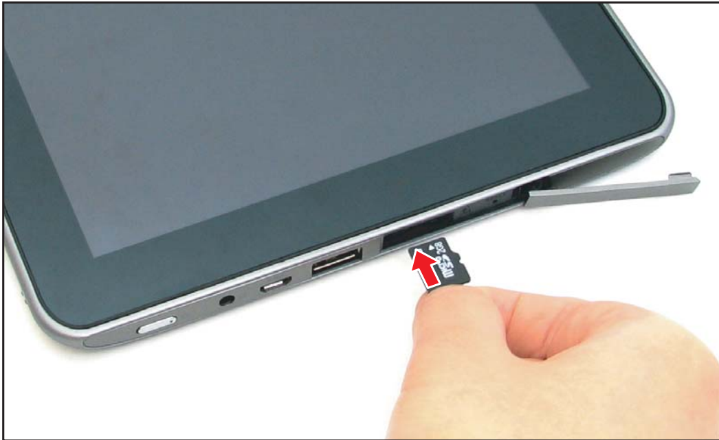
Figure 5-6. Installing the SD Card
