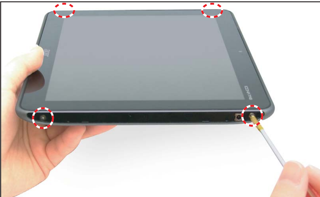
Figure 5-14. Removing the Screws
