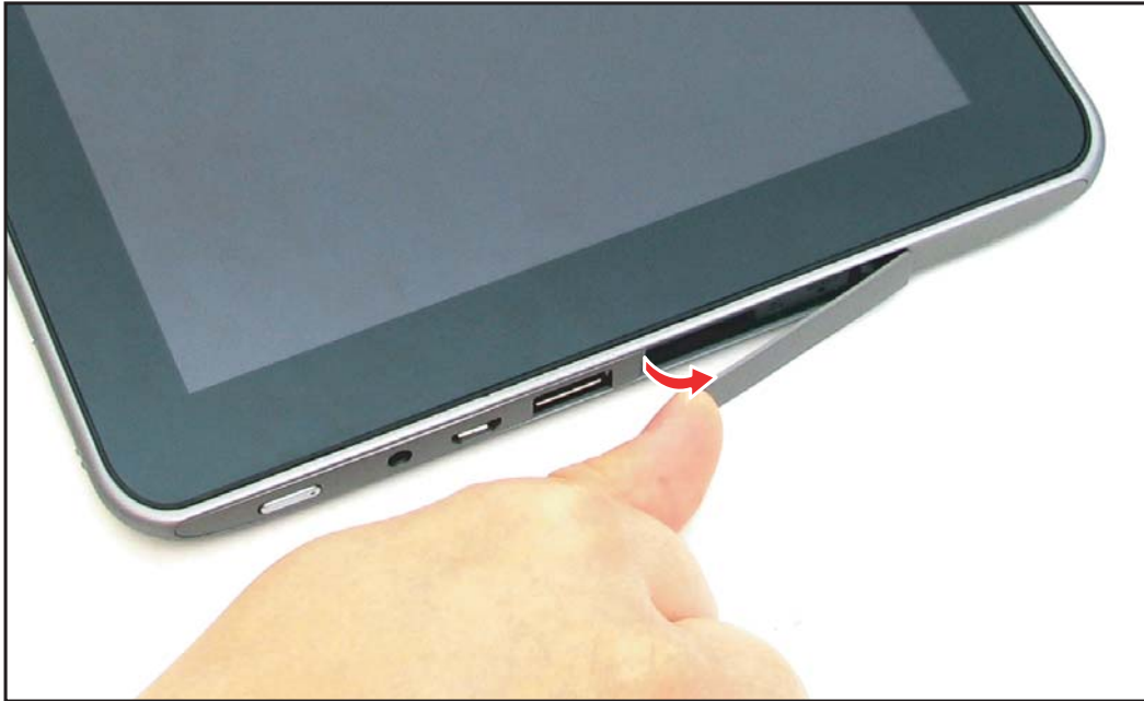
Figure 5-3. Opening the SD Card Cover
