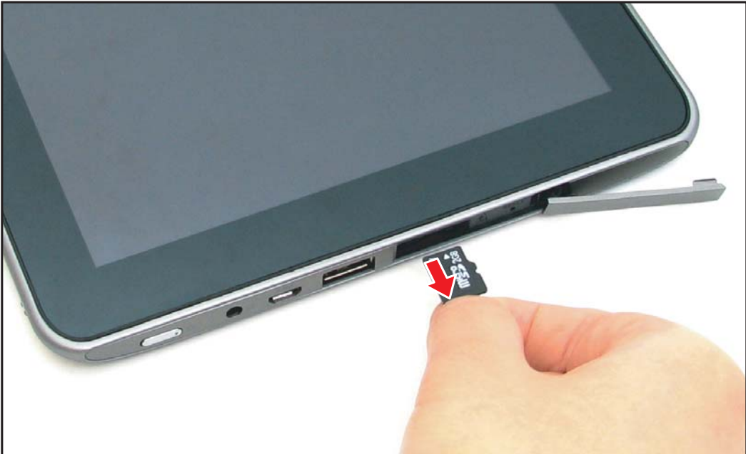
Figure 5-4. Removing the SD Card
