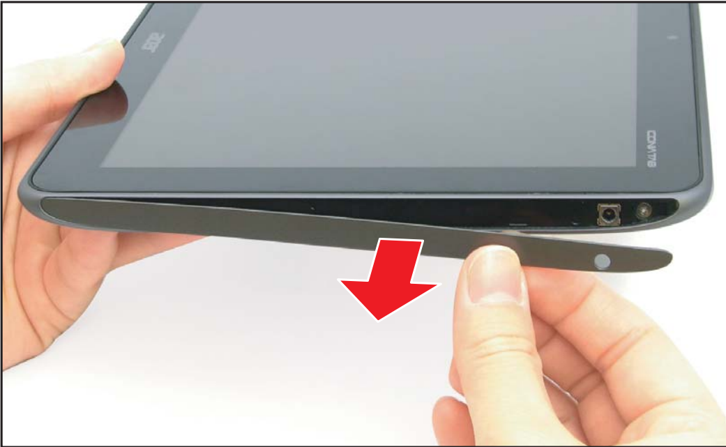
Figure 5-13. Unlocking the Right IO Cover Latches (2 of 2)
