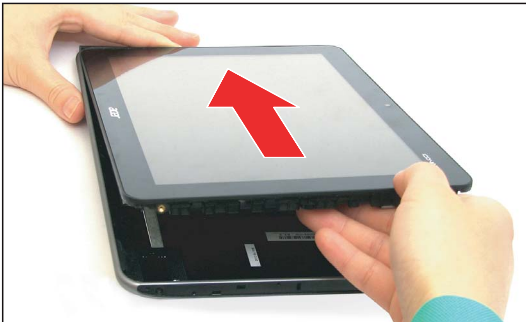
Figure 5-20. Installing the Lower Case (1 of 4)
