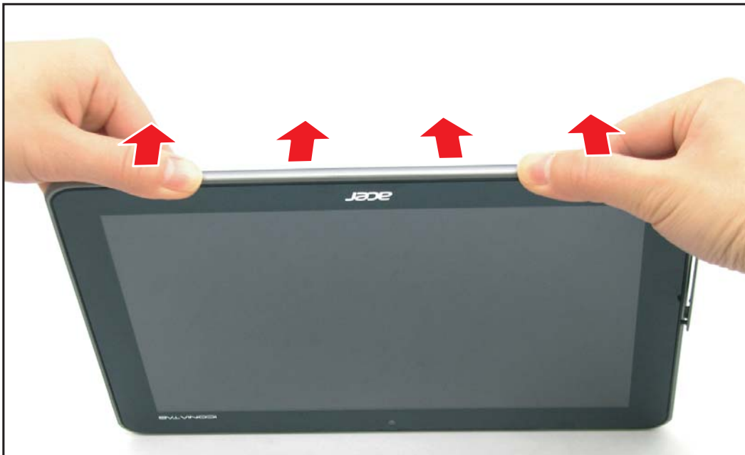
Figure 5-16. Releasing the Side Latches (2 of 4)
