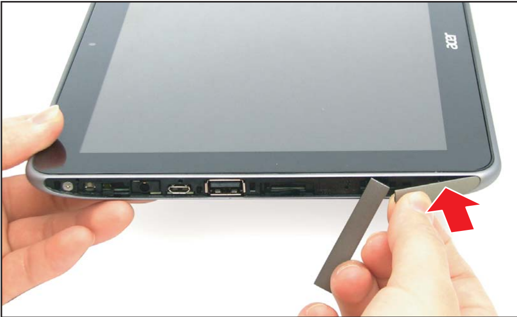
Figure 5-25. Installing the Left IO Cover (1 of 2)
