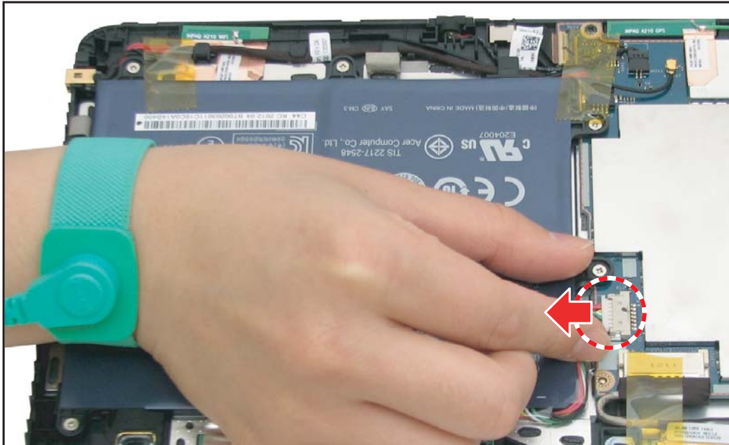
Figure 5-28. Disconnecting the Battery Cable
