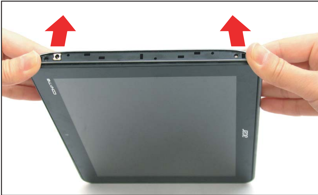
Figure 5-17. Releasing the Side Latches (3 of 4)
