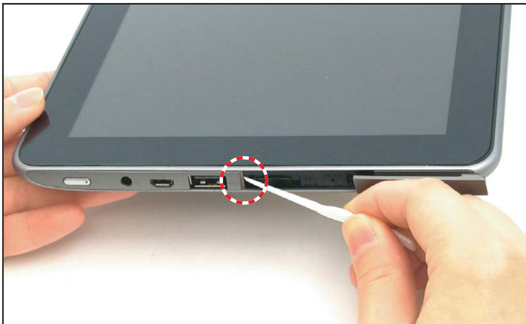
Figure 5-8. Unlocking the Left IO Cover Latches (1 of 4)
