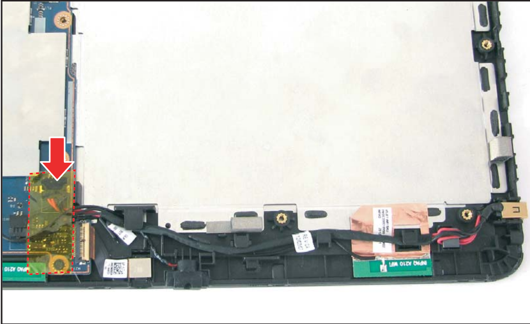
Figure 5-39. Installing the DC-In Cable (3 of 3)
