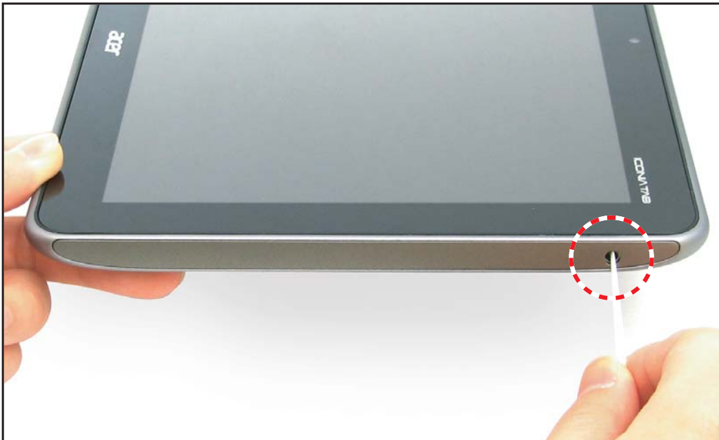
Figure 5-12. Unlocking the Right IO Cover Latches (1 of 2)
