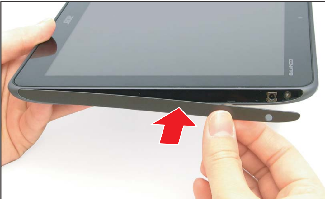
Figure 5-24. Installing the Right IO Cover
