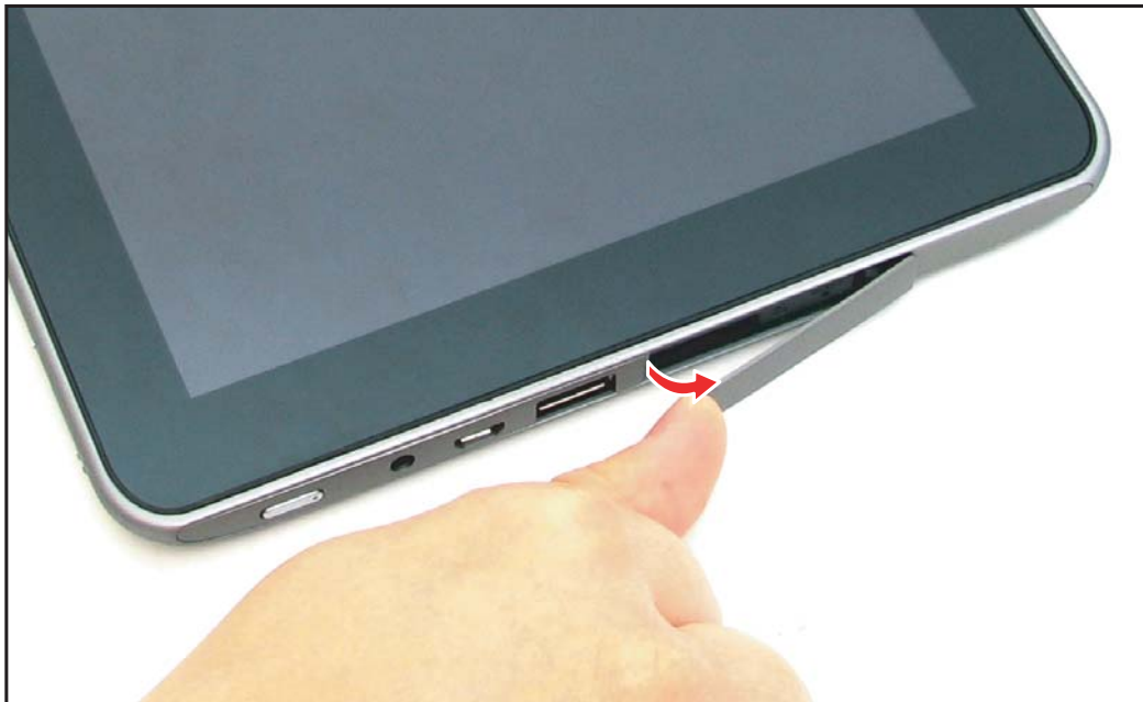
Figure 5-7. Opening the SD Card Cover
