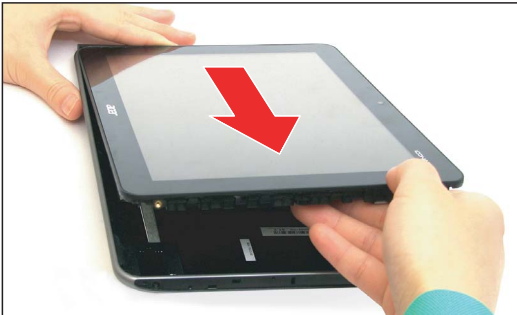
Figure 5-18. Releasing the Side Latches (4 of 4)
