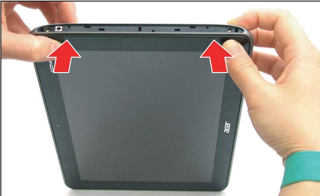
Figure 5-22. Installing the Lower Case (3 of 4)
