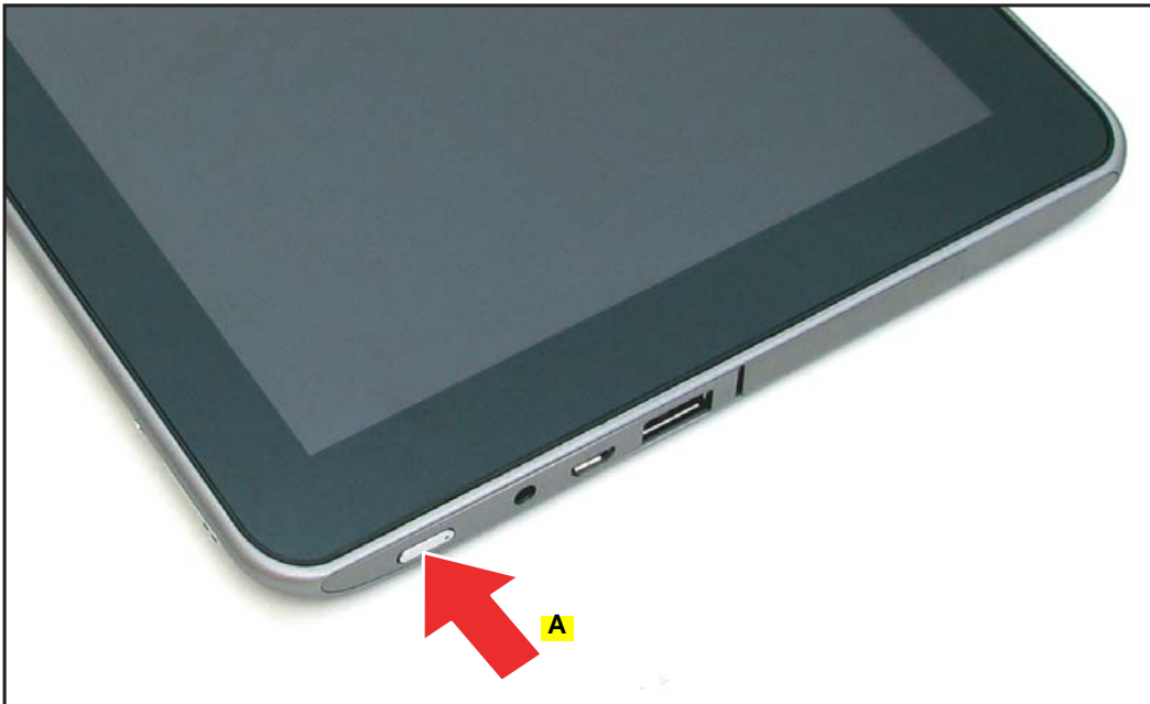
Figure 5-2. Device Overview with Power Button
